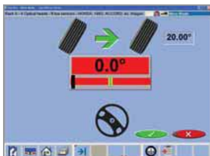
Toe-out on turns measurement
